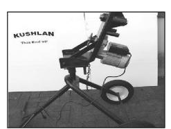
**Step 5.** Install Gear Box Frame with 5/8"  $\times$ 10" Pivot Pin.
