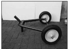
Step 1. Insert Axle in Lower Wheel and Install Wheels.
