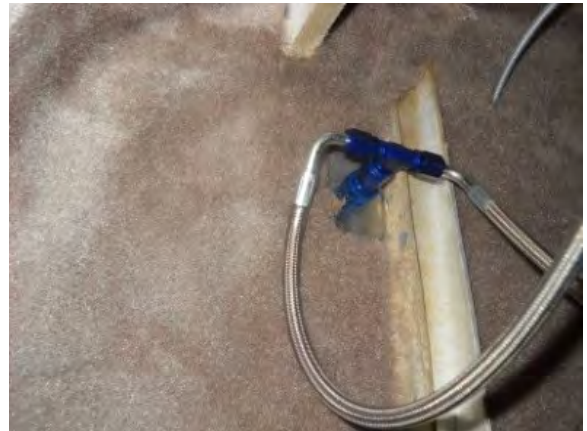
New Bonaco firewall bulkhead fitting and lines
