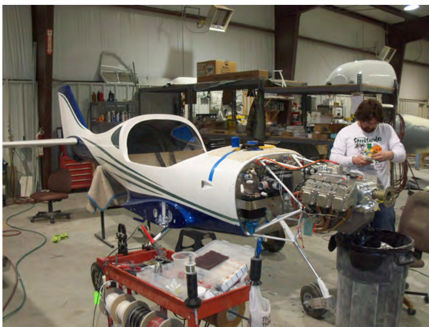
Bryan helps with firewall forward wiring.
