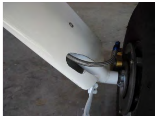
Bonaco brake line exiting the fairing and attaching to the Matco brakes.
