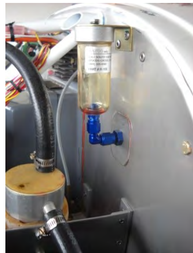
Brake reservoir (provided in the kit from Matco) with Bonaco firewall bulkhead fittings
