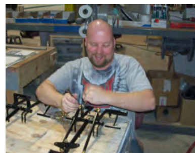
Ronnie installs the master cylinders onto the rudder pedal assembly
