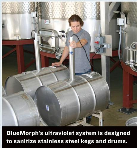
**BlueMorph's ultraviolet system is designed to sanitize stainless steel kegs and drums.**
