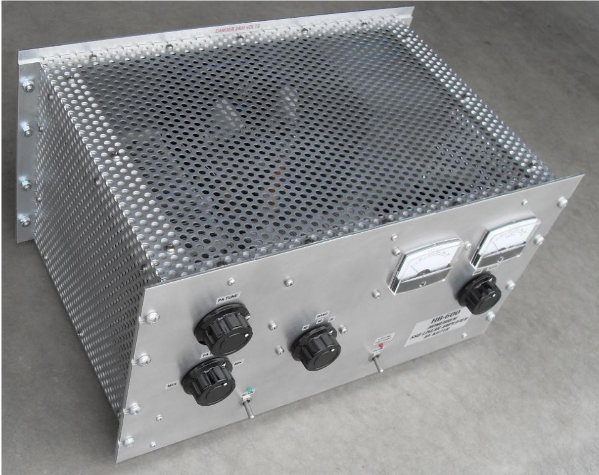
Figure 3: Perforated Sheet Metal Covers Make a Sturdy Box Structure
