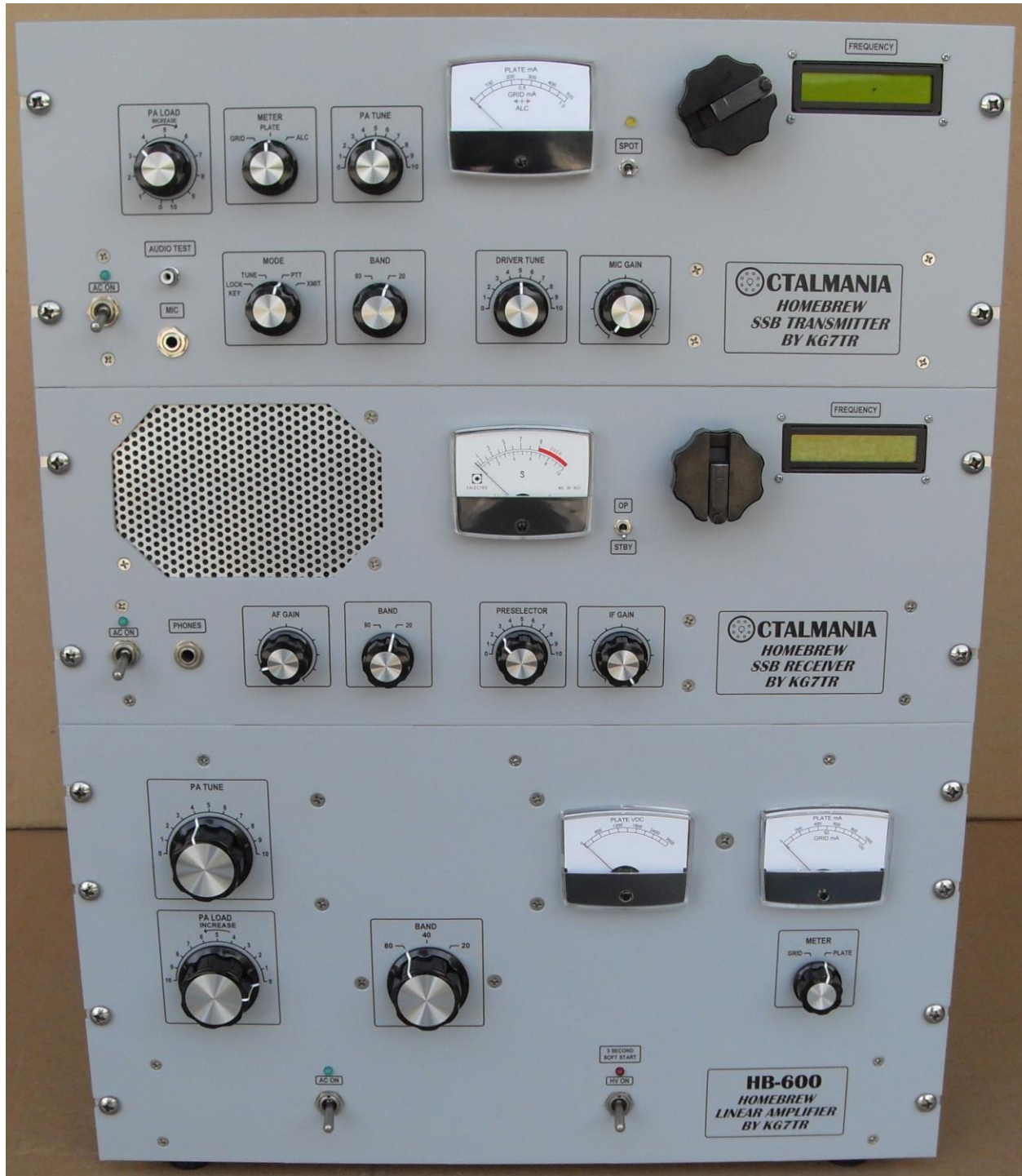
Figure 4: HB-600 with OctalMania Radio Set Stacked On Top. A 25 Inch Tower of 100% Homebrew, Hollow-State SSB!
