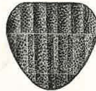
Cross-section at grip of bow after the stave has been worked down to proper size. The grain is perfectly straight, a trait common only to the finest of selected Tonkin butt-cane.
