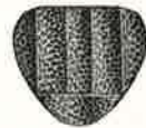
Another cross-section, this one midway between the grip and the nock. Note the perfect uniformity of the bamboo's strong tough fibres.
