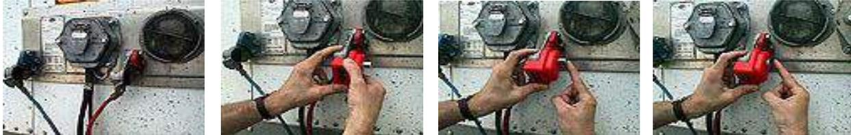
The glad hand lock is applied to the emergency brake (red) connection of the trailer.
