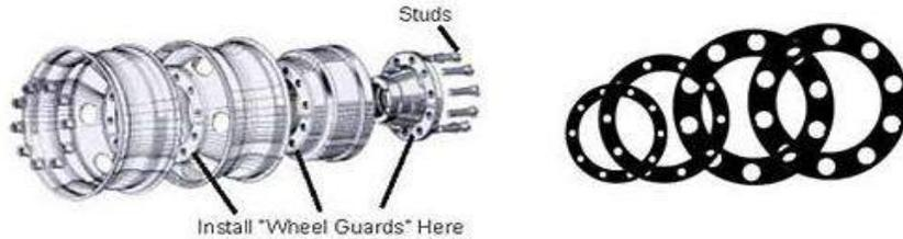
The Wheel-Guard Separator Plate is approximately .040" thick. It is placed between the hub or drum and the wheel, and/or between two wheels in dual applications. Both aluminum and steel wheels can benefit from the Wheel-Guard.
