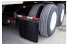
Professionally engineered with each vertical bar of the Aerodynamic flap molded with a patented, curved, wing-type design that makes contact with the water and channels it to the small dead air space on the back side of the flap which form drops that gravitate to the ground. Reduces splashing, and lets air pass through keeping flaps from flapping around at high speeds.
