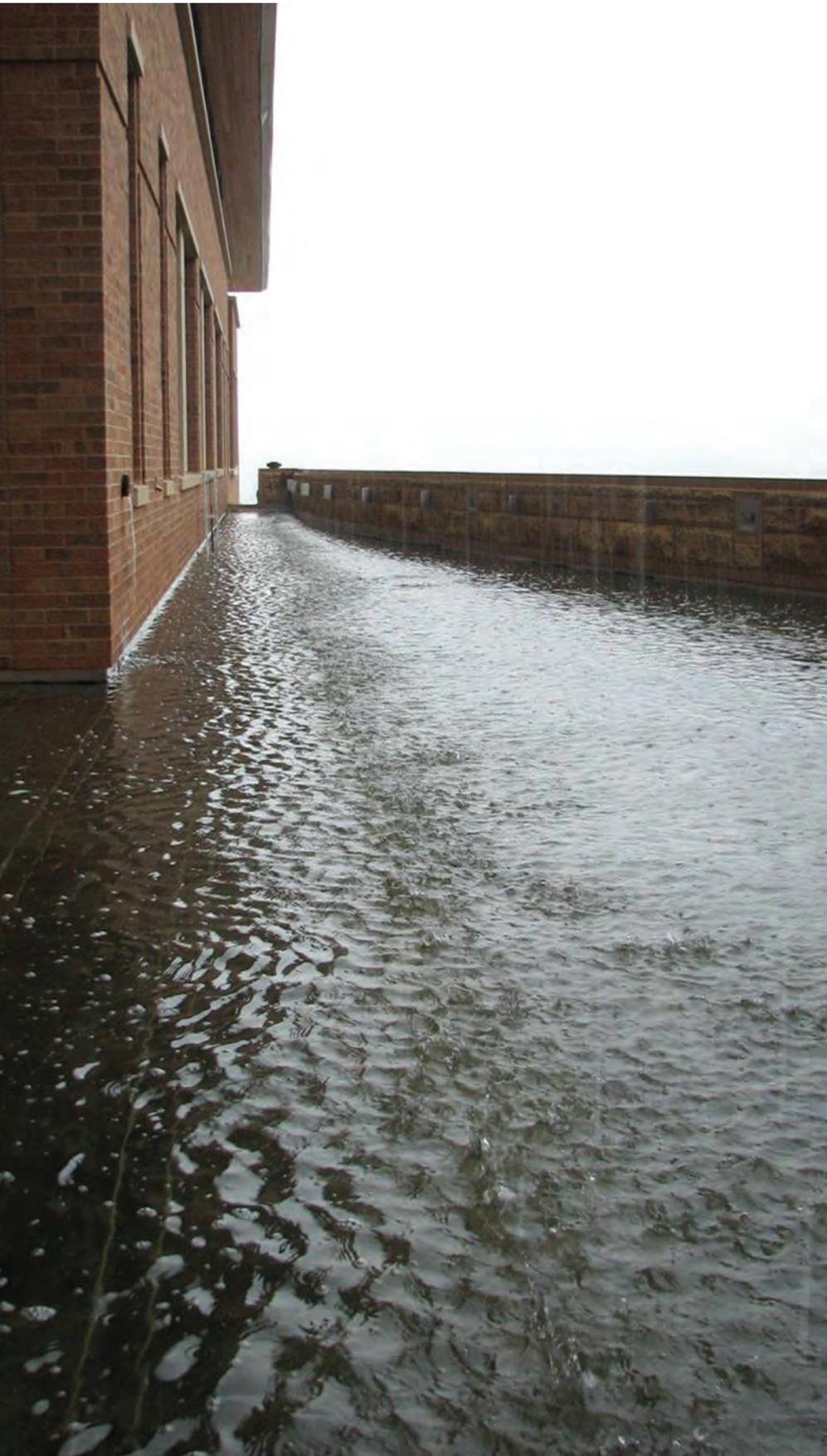
waterproofing system. Decks without significant slope (such as plaza decks) can be tested with a flood test or a flowing-water test. Decks with significant slope (such as parking garage ramps) can be tested using a flowing-water test. Determining a deck's structural capacity is a designer's responsibility.
