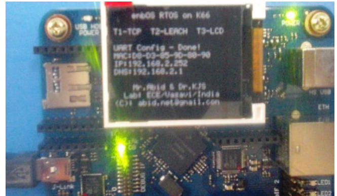
Figure – 4: MCU Gateway configured with static IP
