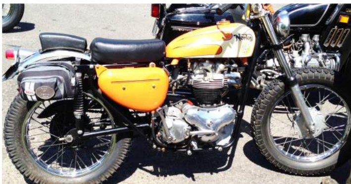
Theo Battaglia's Scrambler (mixed breed): 1959 Norton Dominator 37 ci engine, Matchless G1L frame, Triumph rear wheel, AJS gas tank, N15 Norton Oil Tank, Bater front end, with a headlight from a 1937 Dodge car.
