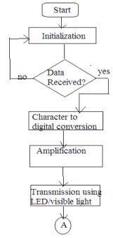
Fig.3: Flow Chart of Transmitter side
