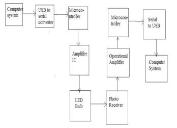
Fig.5:Data Flow Diagram Of Li-Fi Data Transmission
