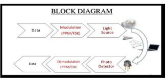
Fig.1: Block Diagram of Li-Fi Technology
