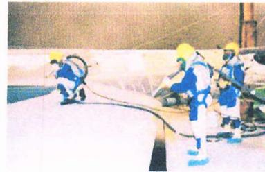
The dry medium, according to Brian Koehl, B-1 structural engineer, is Magic 2 — a nano-composite mix of blended plastics, each having different densities and cutting qualities. He said the texture is like sand grains.
