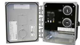
Each unit includes a UL Approved, 240V Power Control Panel complete with Class A Human Rated GFCB, 24 Hour Mechanical Timer, Surge Protector, and 24 Hour Timer for the optional lights. NEMA Type 3r/4x Thermoplastic enclosure.
