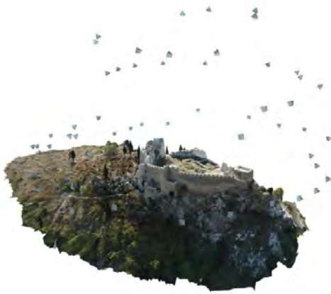
Fig. 12 Position of the drone while taking photographs. Drone circled on 3 different heights around same centre point in fortress
