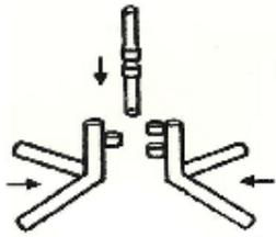
1. Place two halves of the support legs together and insert pivot tube through the center of the legs to join together. (Figure 1)
