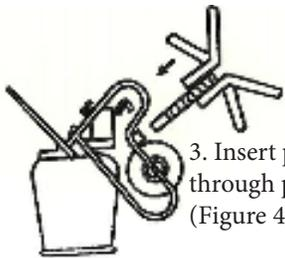
3. Insert pivot tube of pedestal stand assembly through pivot mount and tighten thumbscrew. (Figure 4)
