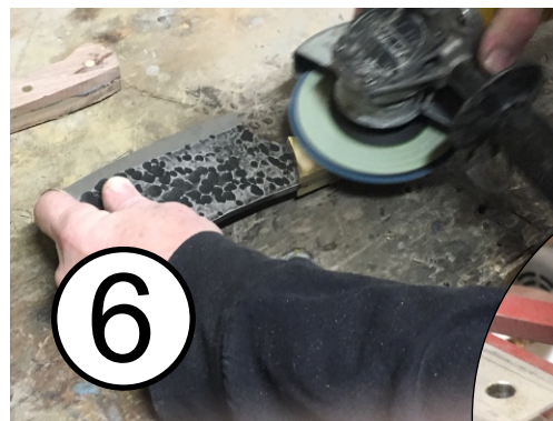
The author using an OBM Small Wheel attachment on 2x72 grinder.
