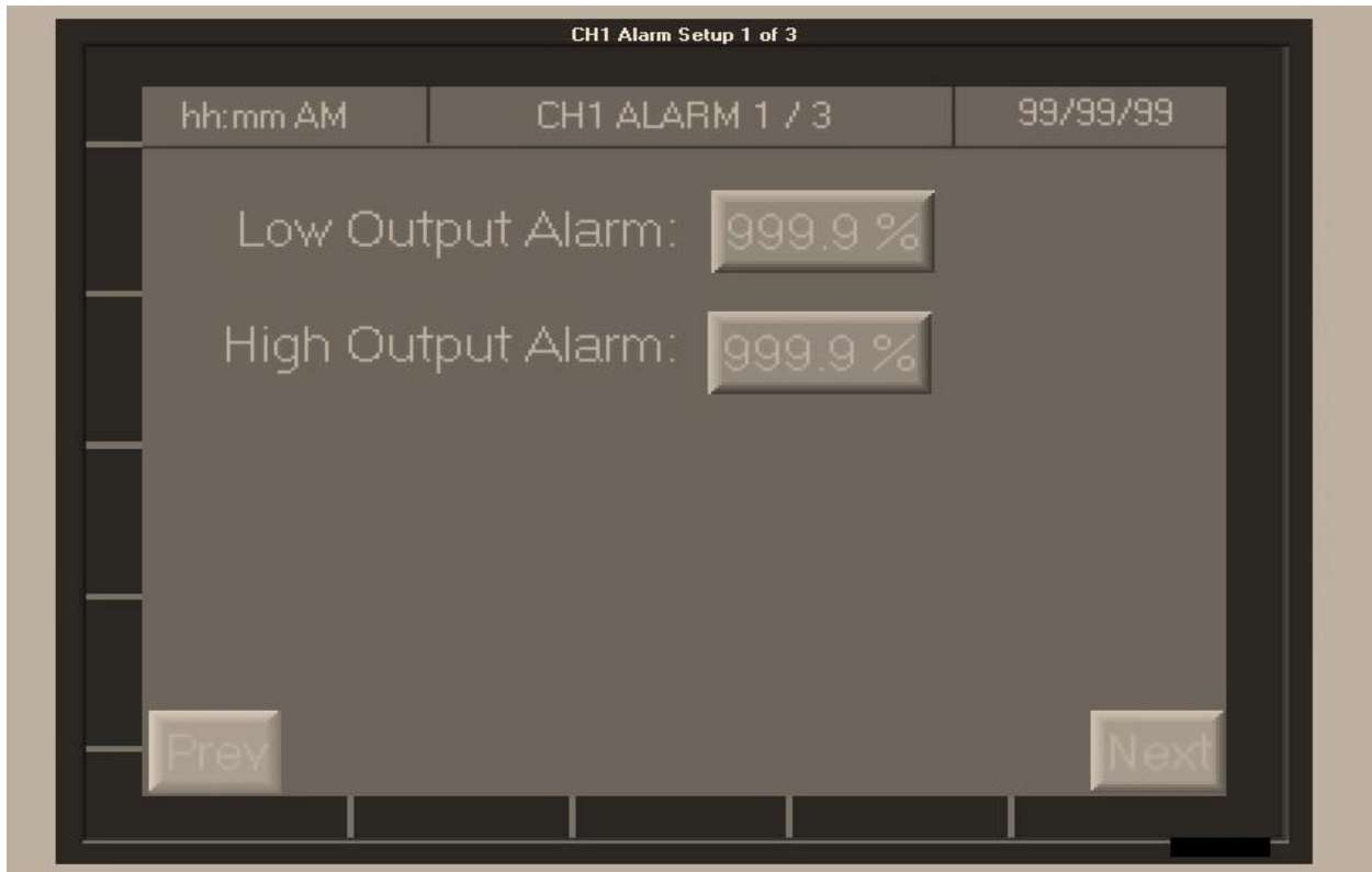
Figure 17: NTL Alarm Setup Screen 1 (of 3) – Feeder Output Alarm Settings
