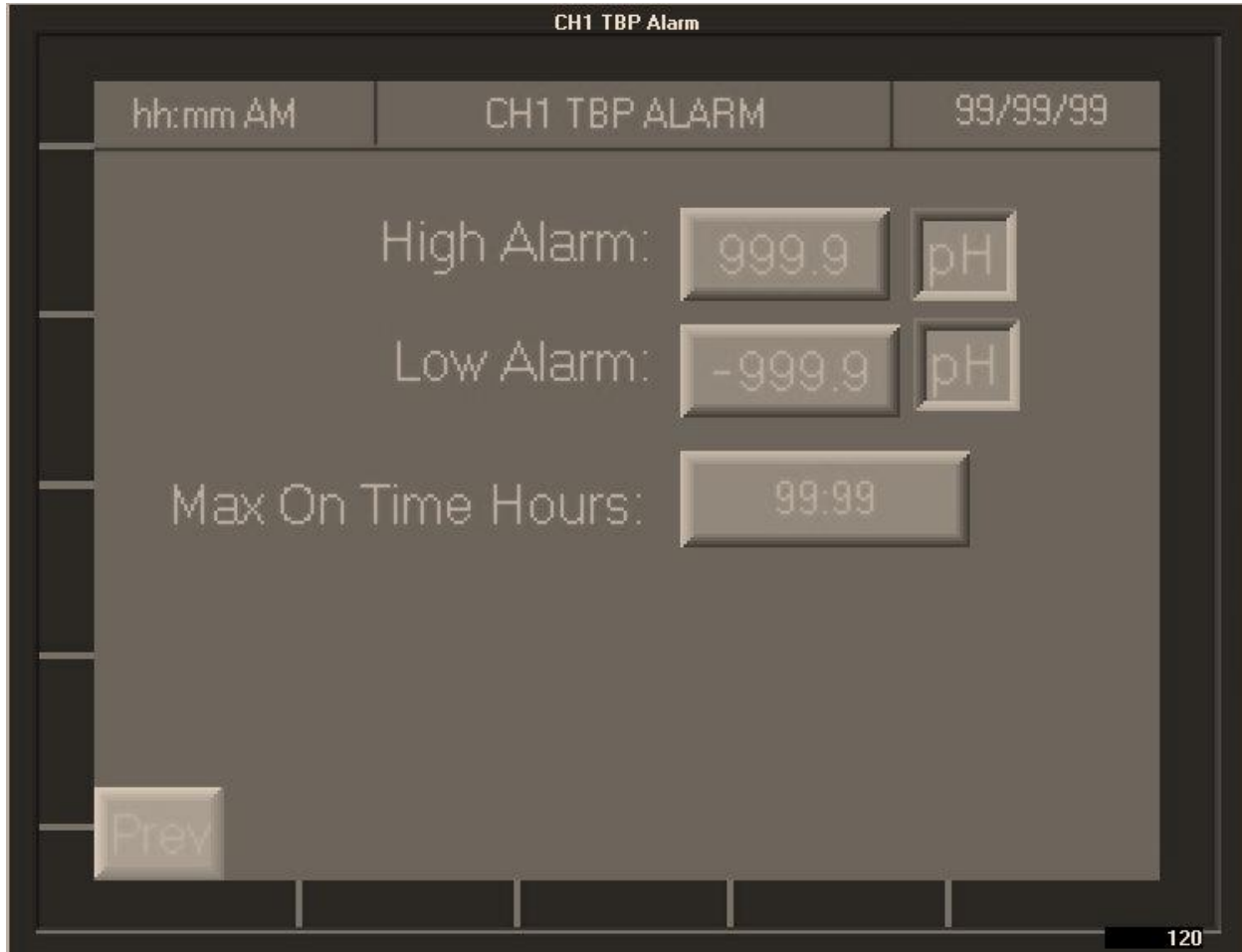
Figure 12: TBP Alarm Setup Screen
