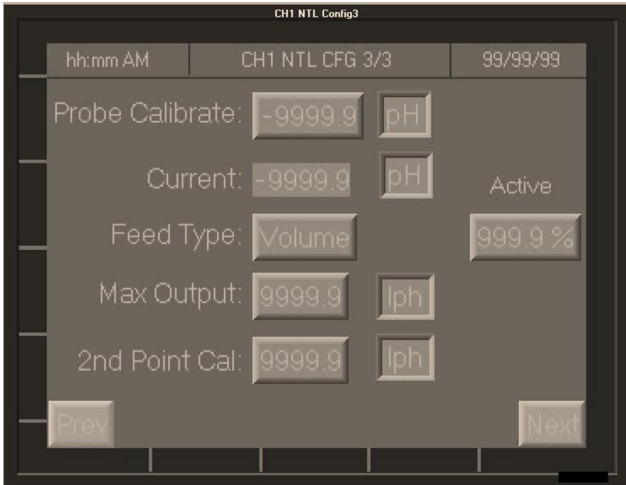
Figure 16: NTL Mode Configuration Screen 3 (of 3)
