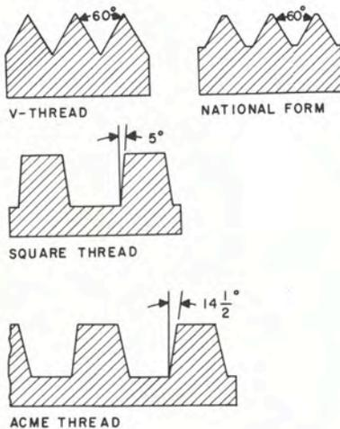
Fig. 5-1. Forms of Common Screw Threads.
