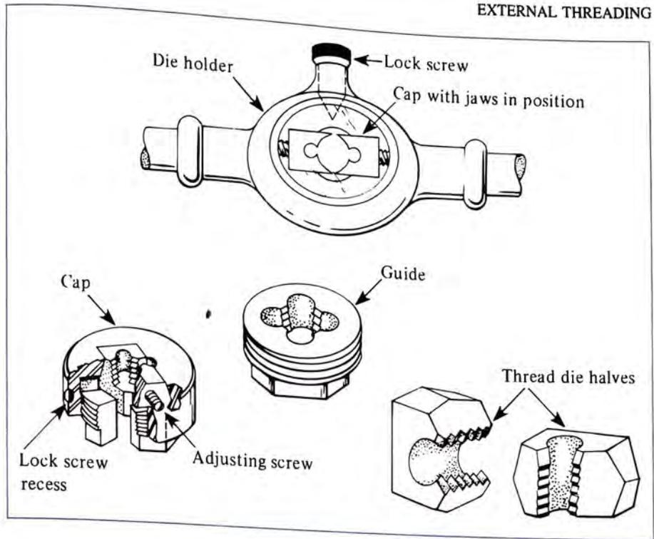
FIGURE 14-8 Features and Assembly of Die Halves, Guide, and Cap
