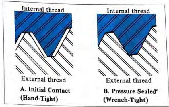
FIGURE 13-15 How Dryseal Pipe Threads Produce a Pressure-Tight Seal
