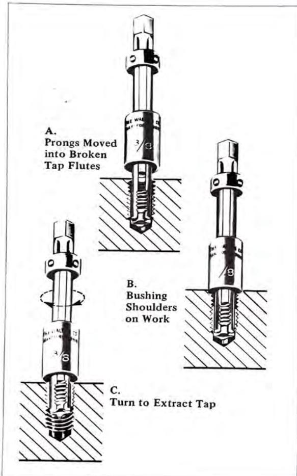
**FIGURE 13-21** Application of a Tap Extractor
