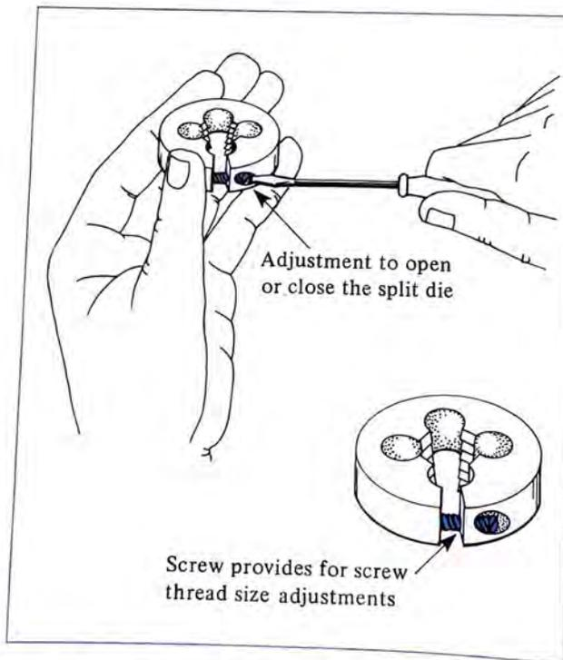
**FIGURE 14-7** A Split Threading Die with a Screw Adjustment
