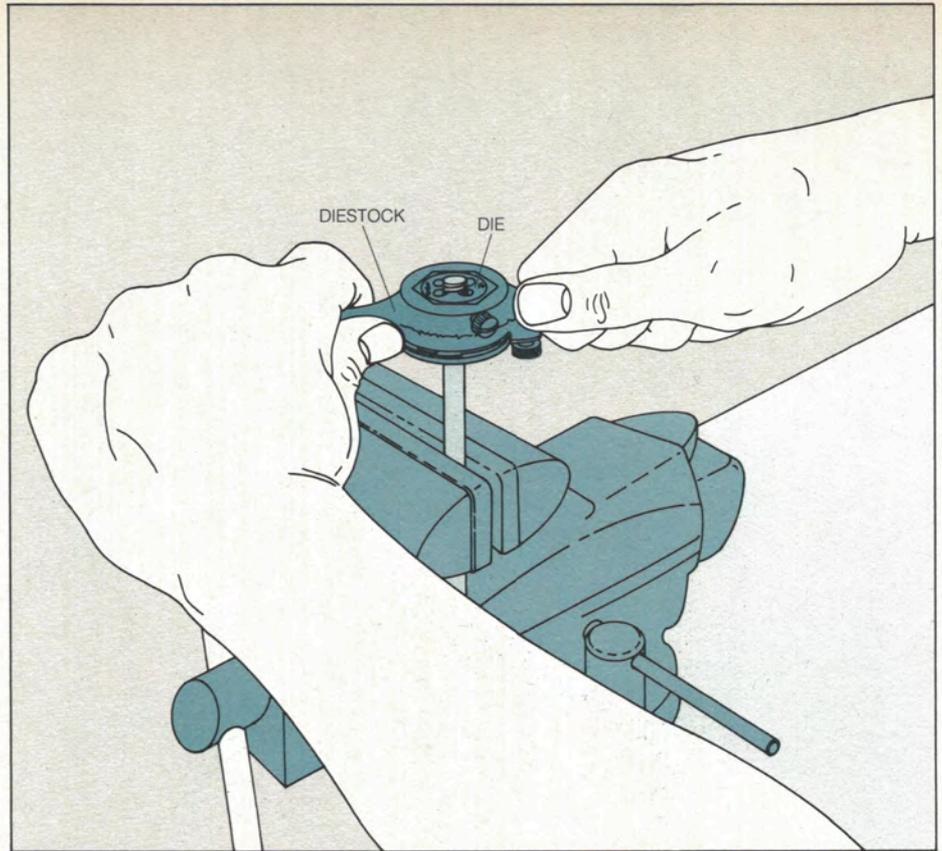
**5 Finishing the threads.** Move your hands to each edge of the diestock and continue threading the rod with a steady motion, backing up a quarter turn to half turn every two full turns, to snap off metal chips. When the guide reaches the mark showing the desired end of the threads, back the die slowly off the rod. Turn the diestock over, put it back on the rod and cut the remaining threads to reach the scratch mark. Clean away any metal chips.
