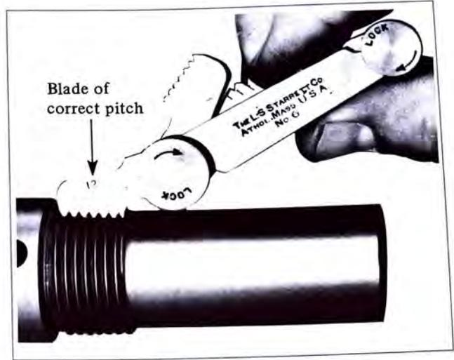
FIGURE 14-3 A Screw Pitch Gage Used to Determine Thread Pitch
