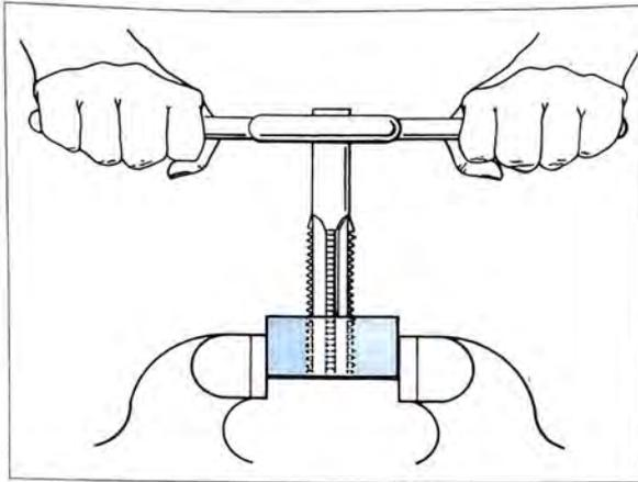
**FIGURE 13-20** Tapping with a Straight-Handle Tap Wrench
