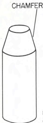
Fig. 5-9. Chamfered End of a Rod.
