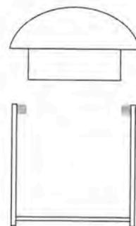
interior wall that fits inside this rim) is soldered onto the lid so that it projects several millimeters into the box.
