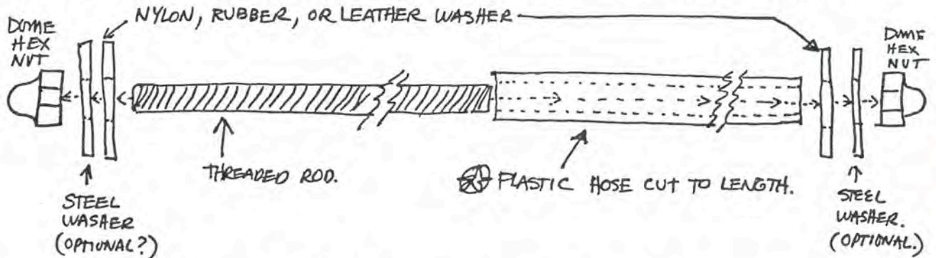
⊗ PLASTIC HOSE MIGHT BE USED TO ALLOW THREADED ROD TO PASS THROUGH CERAMIC PARTS AND KEEP THIS ROD FROM BREAKING CERAMICS:
