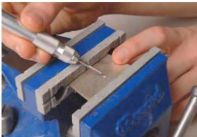
Tap inserted in holder, ready to thread hole drilled with appropriate tap drill
