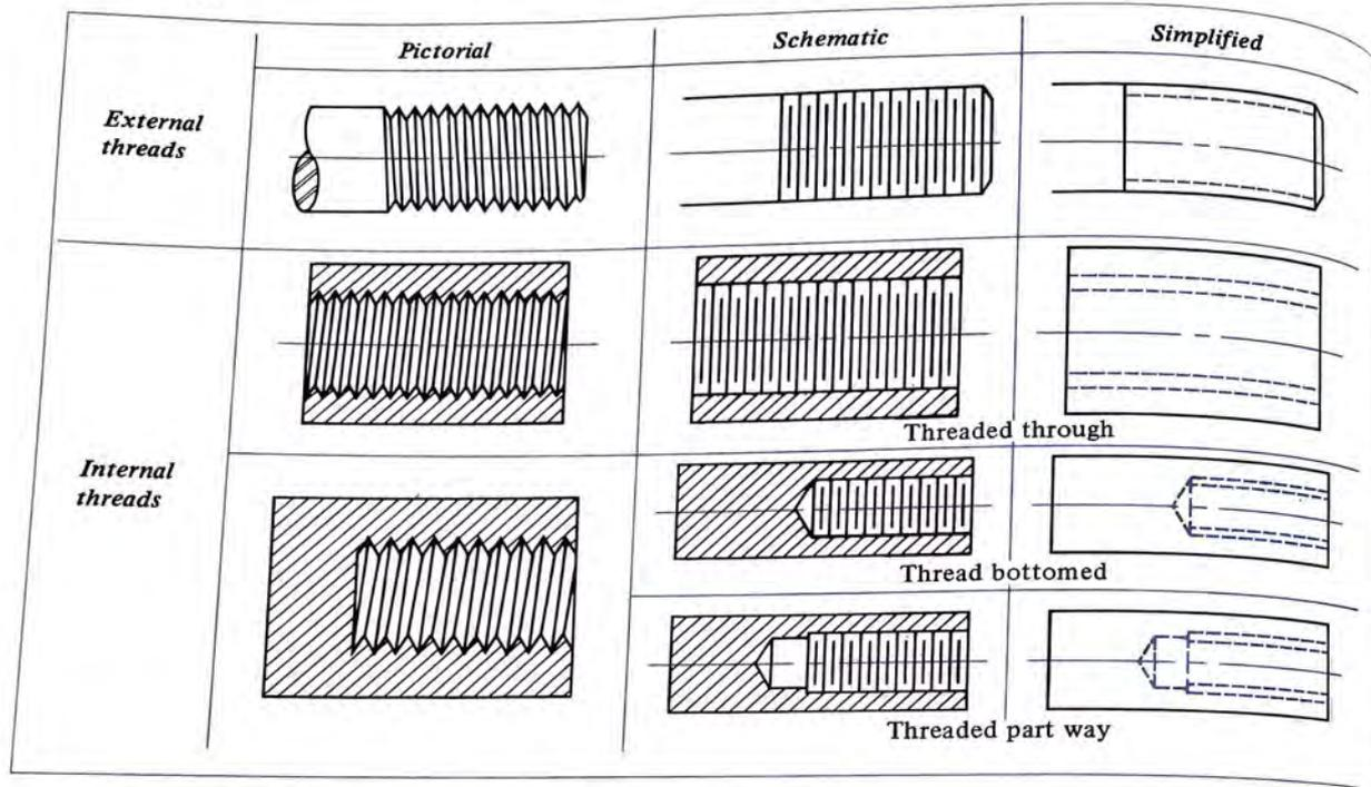
**FIGURE 14-1** Techniques for Representing Threads on a Drawing
