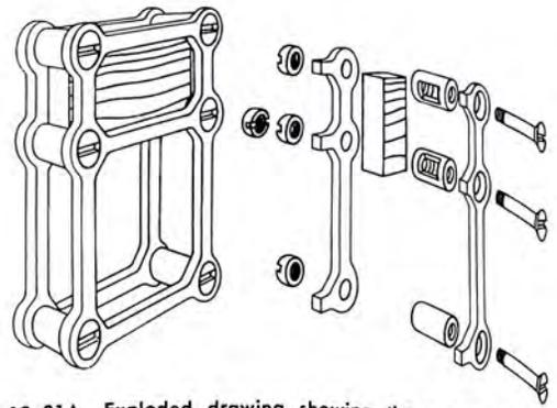
10-31A Exploded drawing showing the parts used in the assembly of the ring at left.
