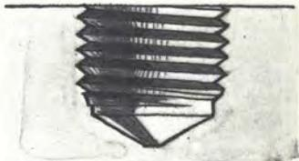
Any stopped holes should be drilled deeper than the required depth of thread because it is impossible to cut right to the bottom. Remove taps frequently to clear them of swarf. Remove swarf from the hole by shaking the work or, where this is not possible, use compressed air (wear safety glasses) or a greased rod. Take care when approaching the bottom of a hole; if you go too far, the tap can easily break.
