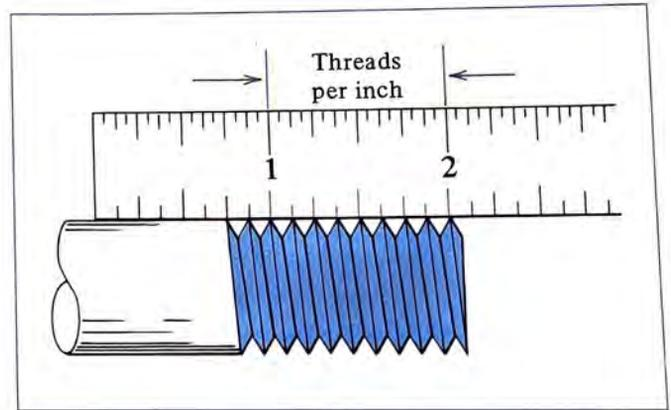
FIGURE 14-4 Using a Steel Rule to Measure the Number of Threads Per Inch
