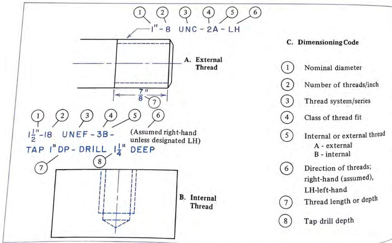
**FIGURE 14-2** Simplified Drawings of Threads, with Dimensions and Dimensioning Codes
