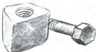
4 Dribble a few drops of oil into the threaded hole to deposit a thin lubricating film on the threads you've just made. Shake off any excess oil.
