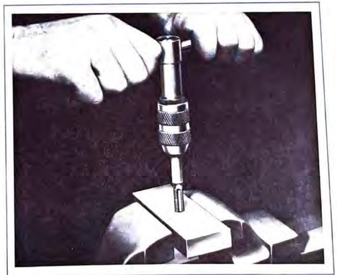
**FIGURE 13-19** Tapping with a T-Handle Tap Wrench
