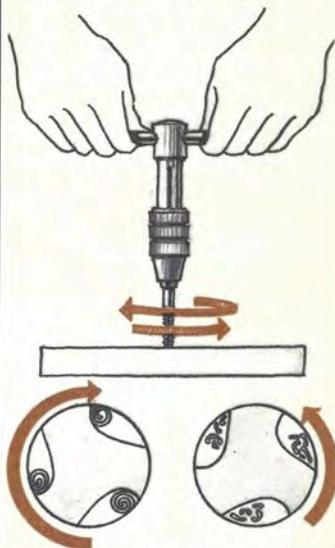
Turn the tap back  $\frac{1}{4}$  turn to break the swarf then proceed with a  $\frac{1}{2}$  turn back and so on.
