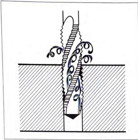
**FIGURE 13-12** Cutting Action of a Low-Angle Spiral-Fluted Tap
