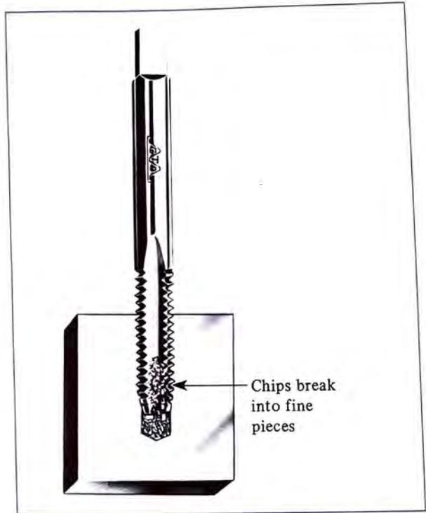
FIGURE 13-10 Cutting Action of a Bottoming Gun Tap
