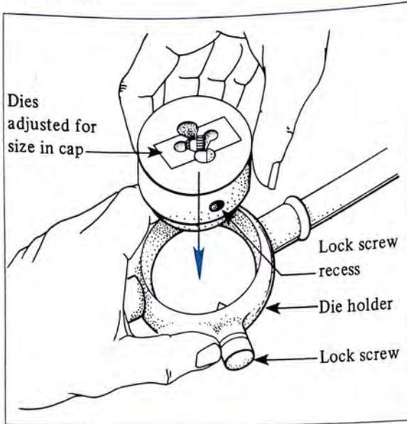
**FIGURE 14-9** Assembling a Two-Jaw Adjustable Threading Die
