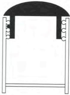
is nothing more than a short finger of metal that will slide along the threaded ramp until the cap is locked into the base. To make a clean and secure joint, drill a hole in the wall of the box, then fit a short length of wire into the hole for soldering. The size of this should match the gap between threads; in this example, it's 16-gauge. The wire is left at a comfortable length for soldering, then trimmed flush on the inside of the lid and cut very short outside. It is
