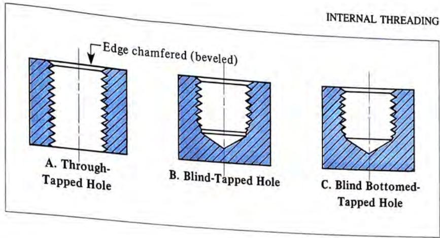
tapped *through* a workpiece (Figure 13-5A). Other holes are tapped part of the way through and are called *blind* holes (Figure 13-5B). Some blind holes are *bottomed* with a thread (Figure 13-5C).
