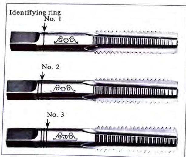
FIGURE 13-8 A Serial Set of Hand Taps
