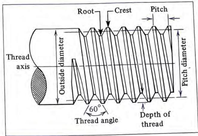
FIGURE 13-2 Basic Features of a Screw Thread
