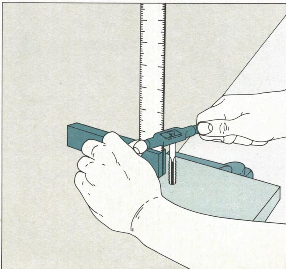
**3 Completing the threads.** When the tap is properly aligned, continue screwing it into the hole steadily and slowly. Do not use pressure; once engaged, the tap is drawn into the hole by its own cutting action. After every two full turns, back up the tap a quarter turn or half turn to snap off metal chips that catch on its cutting edges.
