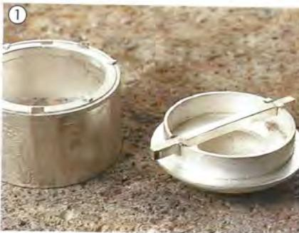
**1** Slots are cut in the inner sleeve to hold the wire tabs of this bayonet catch. The space between the lid and the tab (gray in the drawing) must be slightly smaller than the thickness of the rim that was soldered into the box.
