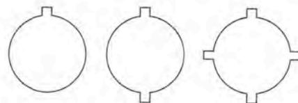
typically small pieces of square wire soldered onto the bezel, but many variations are possible. The catch works with one tab, but two, three or four will also work. If two or more are used, they should be spaced evenly around the lid.
