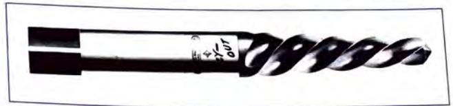
**FIGURE 14-11** Right-Hand Thread Screw Extractor
