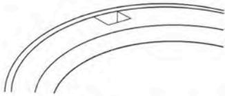
slope on both sides, the lid will tighten by twisting it in either direction.
