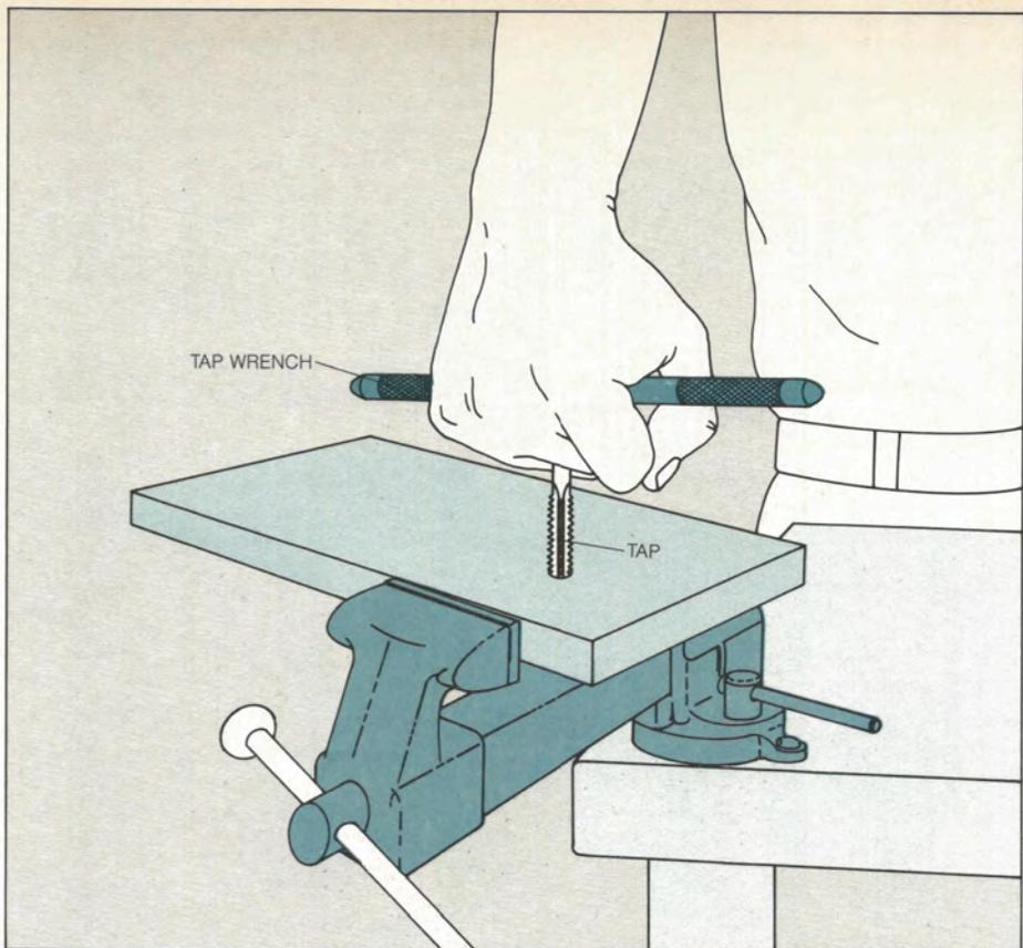
**2 Checking the threads for alignment.** After you have cut the first thread, stand a try square on end about an inch away from the tap, positioning it so that the tap handle will touch the square on the next quarter turn. Grasping the wrench with both hands, step back and sight along the tap and square, to check whether the tap is vertical. If tap and square are not in alignment, unscrew the tap and straighten it.
