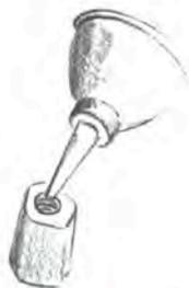
5 Build up a cup with tape around the opening of the threaded hole. This funnel makes it easier to pour melted wax into the hole but, and equally important, the lump of wax here will be a handle that will make it possible to unscrew the rod you are creating. Melt a rigid wax in a can or a spoon, and pour it into the threaded hole.
