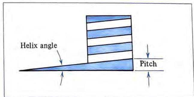
FIGURE 13-1 Early Layout of a Screw Thread
