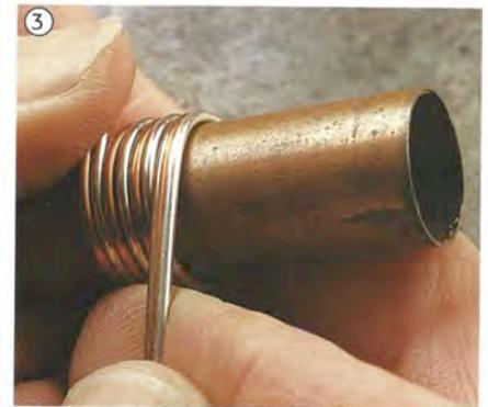
**1** Screw the coil along a piece of metal to make the opening uniform.
