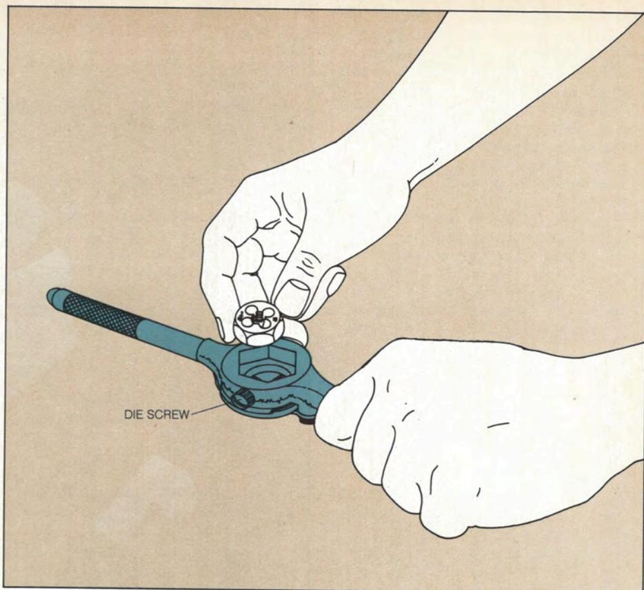
**3** **Beveling the end of the rod.** To allow the die to grasp the rod tightly, file the bevel around the edge of the rod, using a 10-inch half-round medium-coarse file. Grasp the file at either end and, holding it at about a 30° angle, draw it across the edge of the rod, keeping this angle as nearly as possible around the entire edge.
