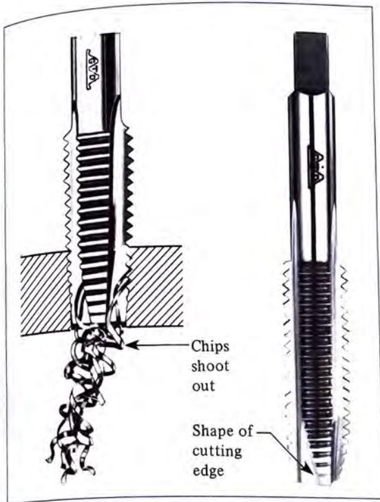
FIGURE 13-9 Cutting Action of a Plug Gun Tap
