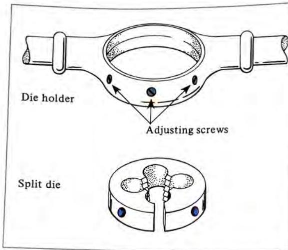
**FIGURE 14-6** Split Die Thread Size Controlled by Three Adjusting Screws
