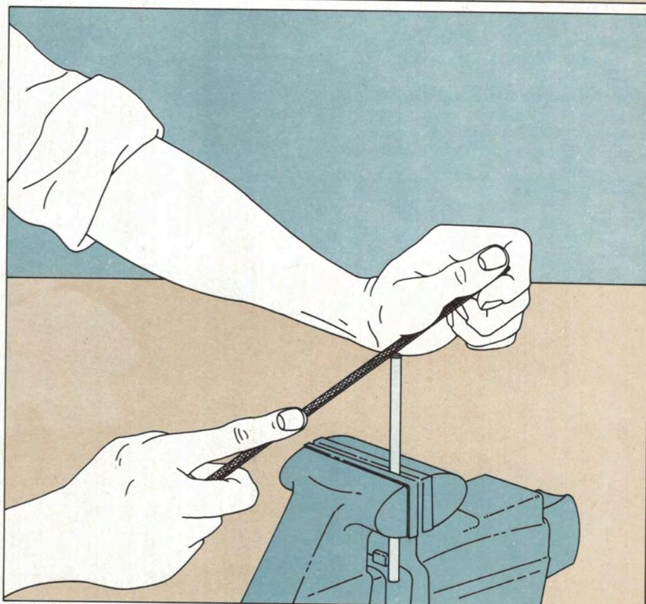
**4 Starting the threads.** Scratch a mark on the rod at the point where you want the threads to end—the depth of the hole into which the rod will fit. Clamp the rod in a vise and place the diestock and die over it, lining up the bottom of the guide with the top of the rod. Turn the chuck plate until the fingers grip the rod tightly; then tighten the screws. Grasp the diestock handles near the die, press down firmly and turn the diestock clockwise to start the threads.
