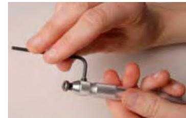
This shows a die being inserted into the handle included in the Reactive Metals set
