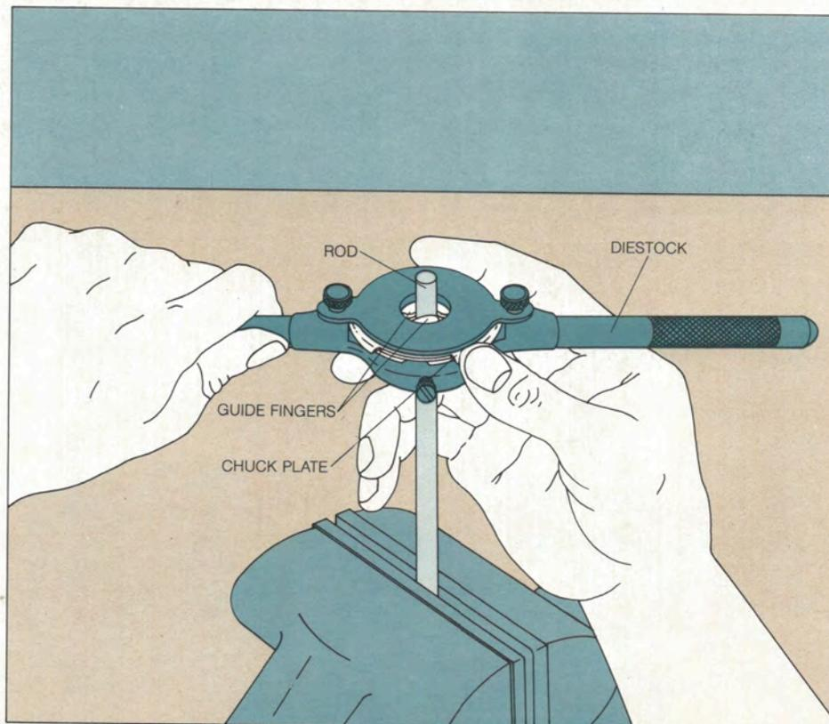
**2** **Inserting the die in the diestock.** Hold the diestock, chuck plate down, and loosen the die screw on the side of the diestock. Insert the die in the depression designed to receive it, placing the tapered end of the die's cutting threads face down, against the guide fingers. Then tighten the die screw.
