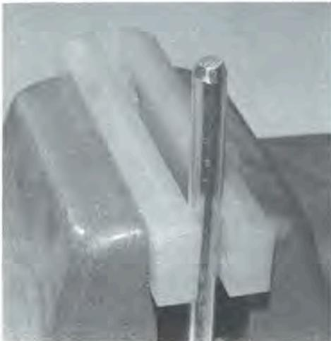
31-4. The end of the silver rod is beveled with a file to allow the die to fit easily over the rod.
