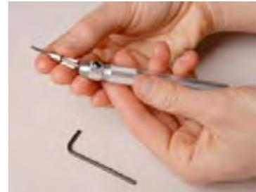
This shows a tap being inserted into the handle
