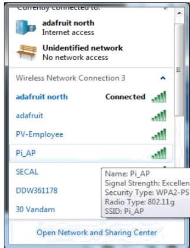
Image(b): Pi_AP named Access Point established
