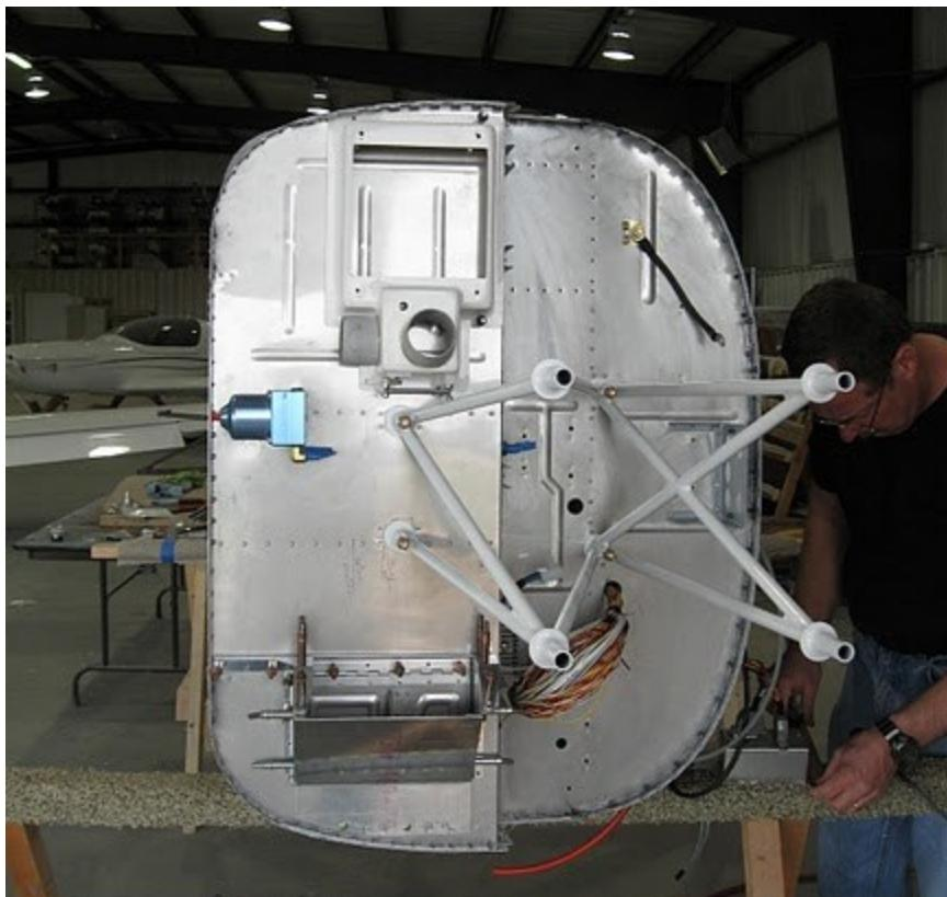
If inserting the bolts from the rear to check for correct length it may be easier to rotate the fuselage onto its side.
