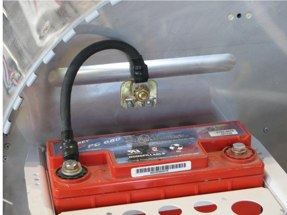
Locate the starter solenoid (this part comes in the Jabiru 2200 engine accessory bag) on the fire-wall in the lower pair of holes in the RV-12 firewall. These pre drilled holes were originally for the Rotax solenoid and the Jabiru solenoid mounts in the same place using AN4-4A bolts and AN960-416L washers. Since the upper pair of holes will not be used install a AN4-4A bolt and AN960-416L washer in each of the holes to seal the firewall.
