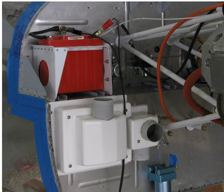
Pre mark four holes on the perimeter of the filter box evenly spaced around the air filter portion of the box. Rivets will eventually be installed at these locations to secure the box to the firewall.
