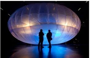
The inflatable part of the balloon is called a balloon swirl(envelope) .Loon's balloon envelopes are made up from sheets of polyethylene plastic and they measure 15m wide and 12m tall when fully inflated. At the time of taken balloon out of the service gas is released from the envelope In the unlikely event that a balloon drops to quickly and parachute attached to the the of envelope is deployed.
