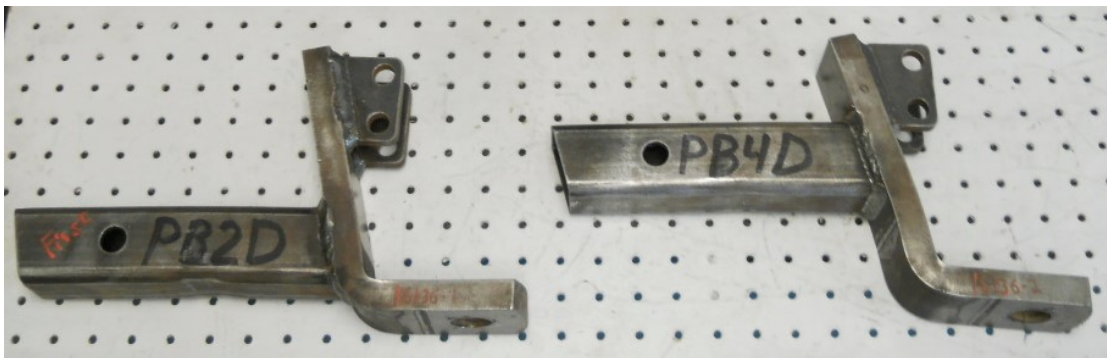
Following Overloads in Step a.– Some Bend in Tube and in Ball Platform
