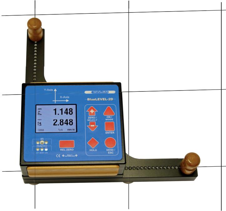
The wylerSPEC software makes it possible to utilize the full functionality of the BlueLEVEL-2D: The measurement values along the X and Y axes are read out simultaneously.
