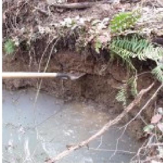
*A test pit with a high water table*
