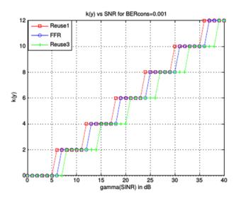
Figure 4 Rate adaptation vs SINR plot
