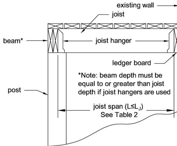
**Figure 2. Joist Span – Non-Ledger Deck.**
