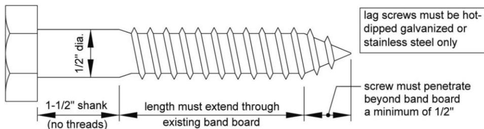
**Lag screw installation requirements:** Each lag screw shall have pilot holes drilled as follows: 1) Drill a  $\frac{1}{2}$ " diameter hole in the ledger board, 2) Drill a  $\frac{5}{16}$ " diameter hole into the band board of the house. **DO NOT DRILL A  $\frac{1}{2}$ " DIAMETER HOLE INTO THE BAND BOARD.**
