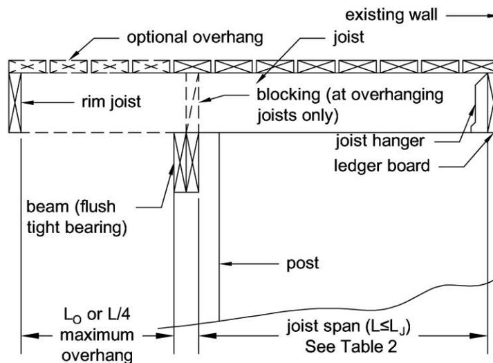
**Figure 1B. Joist Span – Joists Attached at House and to Side of Beam.**
