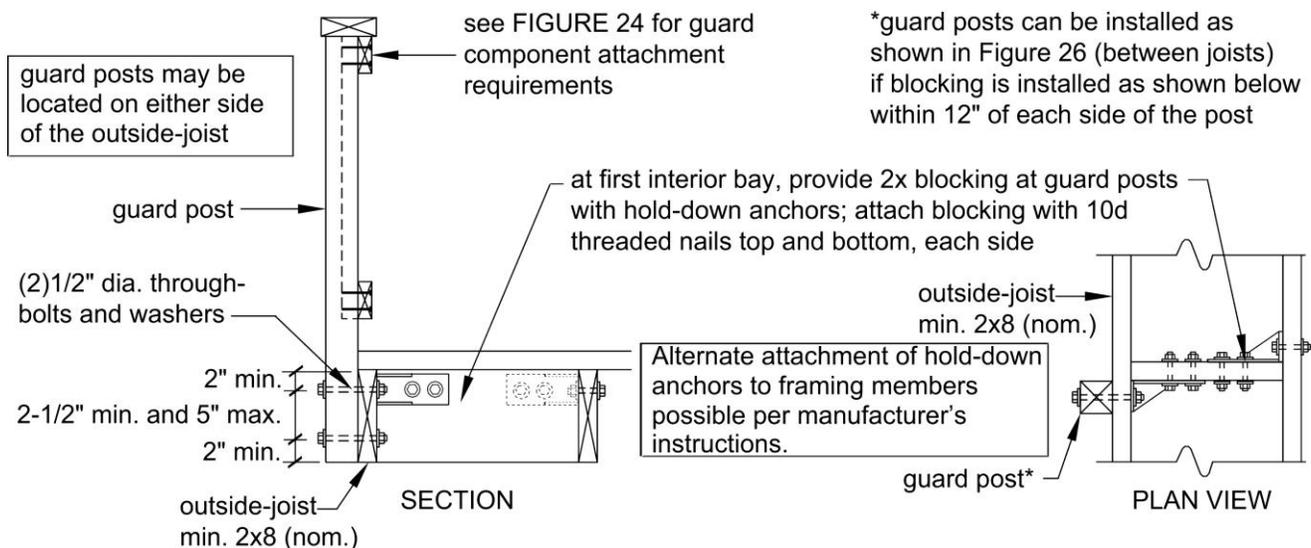
**Figure 26. Guard Post to Rim Joist Example.**
