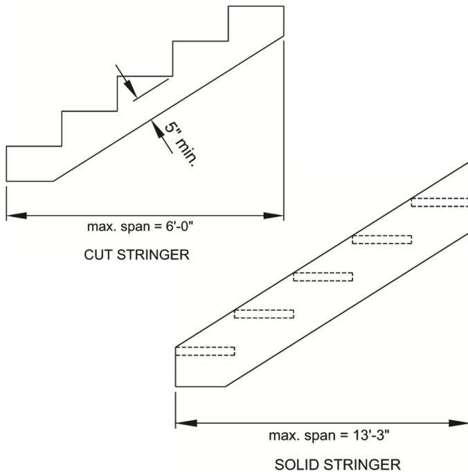
**Figure 29. Tread Connection Requirements.**
