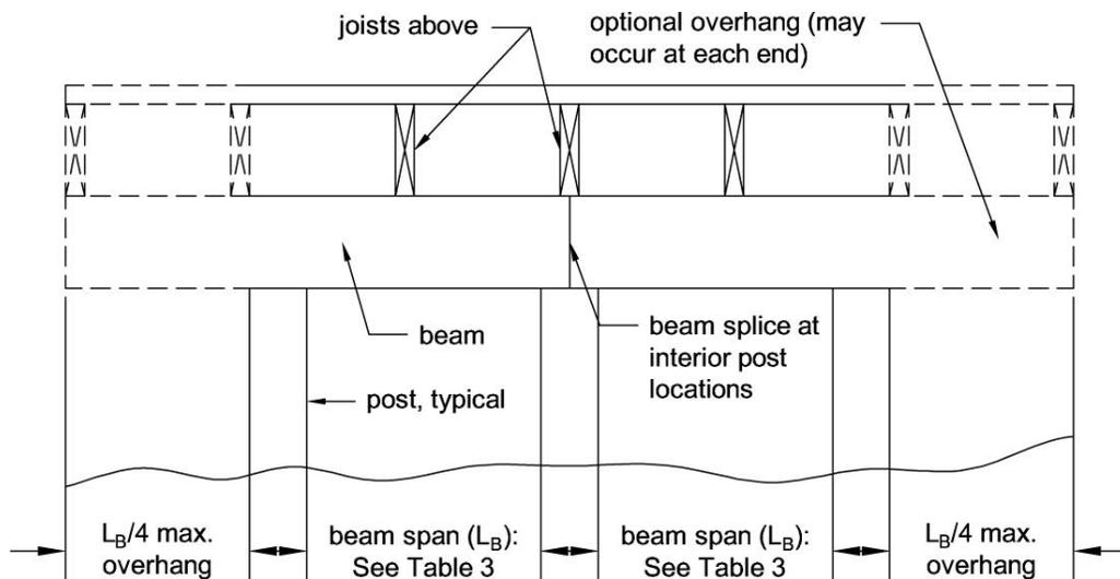
Figure 4. Beam Assembly Details.
