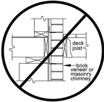
**Figure 18. No Attachment to House Overhang with Ledger.**
