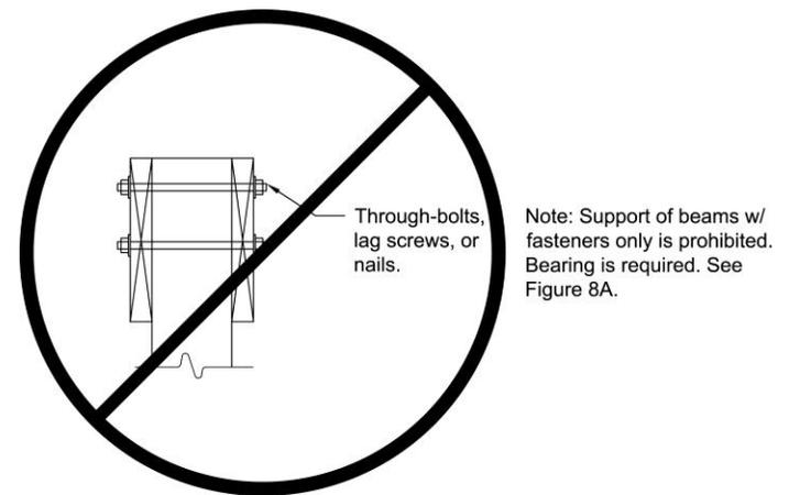
**Figure 8A. Post-to-Beam Attachment Requirements.**
