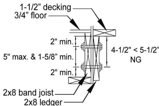
**Table C5. Revised Bolt Spacing Requirements for 2x8 Ledgers to 2x8 Band Joists.**
