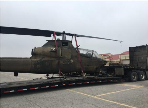
Before that, the pair had to remove all the anachronistic add-ons of its later service, including wire-strike protection devices, and replace the tail rotor and tail rotor gearbox. They also had to replace the AH-1S nose housing, which features the later addition of a swivelling turret.
