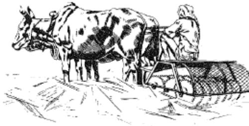
**Fig. 3.** Olpad Thresher, made in India on the pattern of thresher; diameter of discs about 15 cm, number of discs 20.
