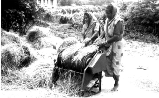
**Fig. 7.** Paddy Pedal Thresher in Operation
