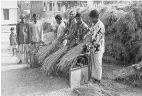
**Fig. 8.** Pedal or Treadle Thresher
