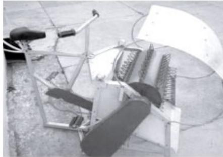
**Fig. 10.** Developed VL Paddy Thresher
