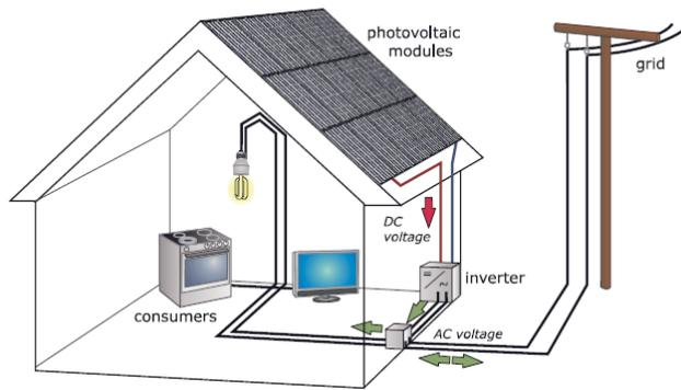
Figure3. Principle of grid connected photovoltaic system.
