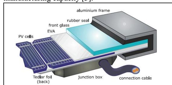
Figure 1. Structure of Photovoltaic Module [1]
