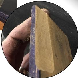
We recommend beveling a scrap piece of wood to confirm bevel width is set accurately.
