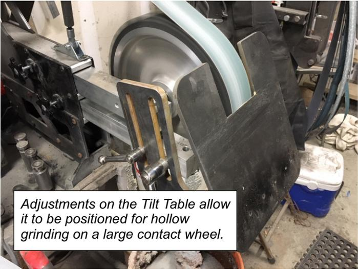
Adjustments on the Tilt Table allow it to be positioned for hollow grinding on a large contact wheel.
