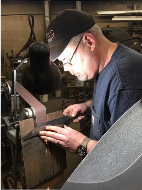
Center Line Scribe used to mark parallel Railroad Track lines on blades edge.
