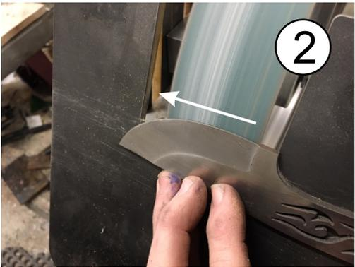
Maintain pressure to keep the blade flat while pulling it horizontally across the belt. As with flat bevels, it's very important to accurately grind evenly up to the scribed lines.
