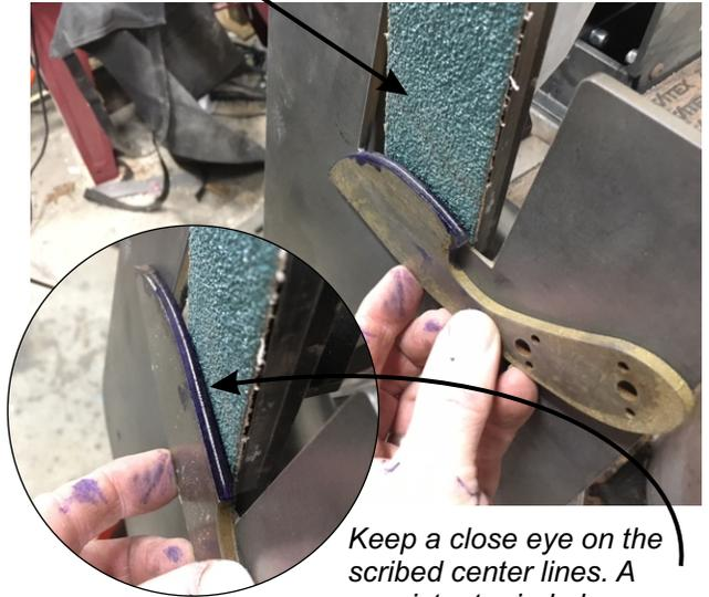
2 Hold the blade flat against the Tilt Table and then slowly bring it up and into contact with the grinders belt. The blade can then be moved horizontally. Its important to keep a little pressure against the blade to hold it flat against the table during all grinding. Use a coarse grit belt to remove the bulk of the material. Then change to a finer grit to finish the bevel.
