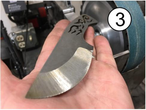
A finer grit belt can be used to polish the bevels.
