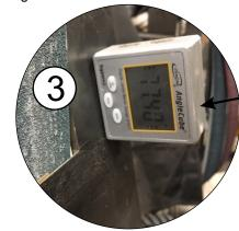
A digital angle meter can be used to reset the Tilt Table to desired angle for post heat treating bevel polishing.
