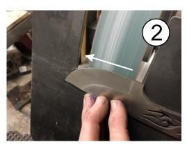
Maintain pressure to keep the blade flat while pulling it horizontally across the belt. As with flat bevels, its very important to accurately grind evenly up to the scribed lines.
