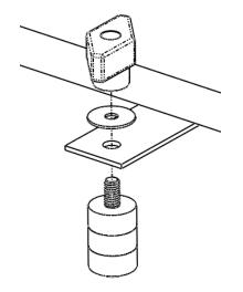
The threads of the Anchor Assembly will fit up into the holes. Replace the Washer and T-Knob. Screw the T-Knob and Washer down until it is finger tight but can still spin freely in the hole.
