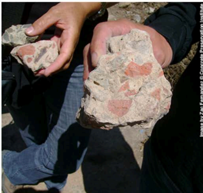
The team has found crushed bricks from an earlier structure used as aggregate in the main cell house. Image by Zac Fernandez © Concrete Preservation Institute
