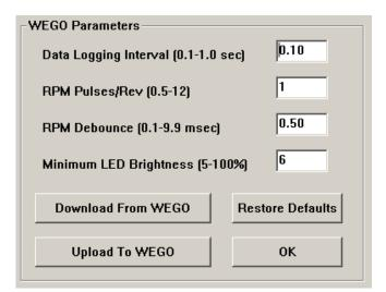
If you are logging engine RPM, you must set the correct value for RPM pulses per revolution (PPR). Some general guidelines follow, based on what type of signal you have connected to the WEGO brown wire:
