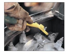
Top access service panel is of sufficient size to replace the cutting bits without raising the planer from the surface or removing the drum.
