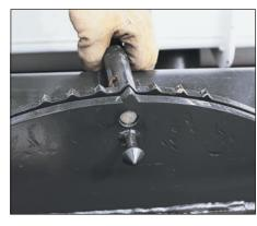
The **planer housing** oscillates  $\pm 15^{\circ}$  for cutting at an angle or matching uneven surfaces. An indicator is provided with markings locating each  $\pm 5^{\circ}$  of oscillation. If desired, it may be put in a locked position to prevent rotation. Hydraulic oscillation standard on 15-in. curb planer.
