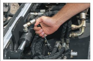
Use the diverter valve control to switch between hydraulic side-shift and hydraulic oscillation.
