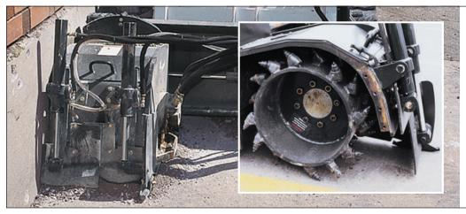
The right ski and end plate are removable to allow flush milling against curb or wall (14", 16", 18" and 24" drum). Side cutting bits decrease drum binding and provide a vertical edge for improving the joint bond.
