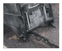
The **ski wear pads** are replaceable and provide consistent depth control by penetrating through debris in the path of travel. Optional planer wheel kit available to replace skis.
