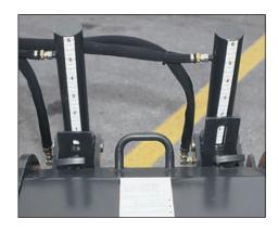
The **depth of the skis** is indicated by a depth gauge visible from the operator's seat.\*\* (Single ski depth gauge on 15-in. curb planer.)
