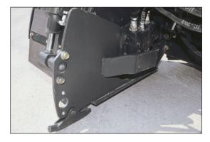
The two-position single ski mount allows the curb planer to be used for milling concrete curbs when mounted in the top hole, or used as a traditional planer for asphalt and concrete when the bottom mounting hole is utilized.
