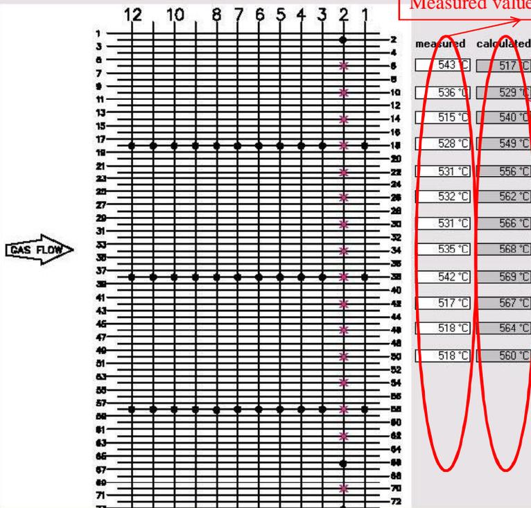
Calculated values based on Geometrical dimensions like
