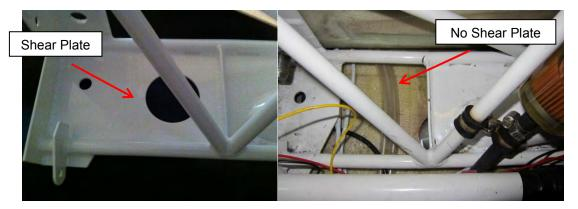
Figure 5, New Spar Box Left Side vs Old Spar Box
