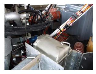
pins so they can't back out. I took a Dremel<sup>®</sup> tool and cut a small slit on either side of the fiberglass inlet cooler shroud where the pins could be angled
