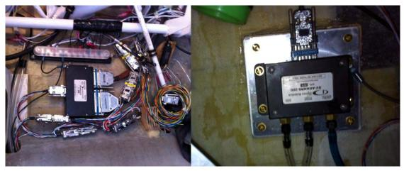
Figure 8: Engine Monitoring Computer (left) and ADAHRS (right).
