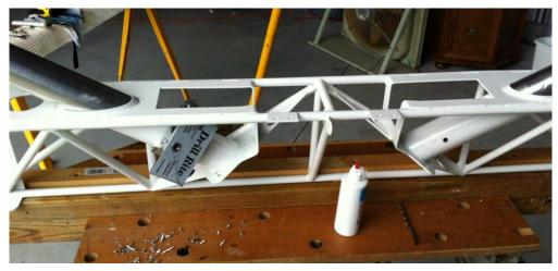
Figure 11: Drilling the gear holes (I used a Drill Rite guide).
