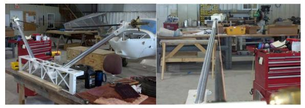
Figure 10: Setting the Toe (Factory pictures)
