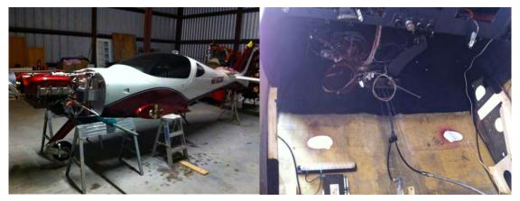
Figure 9: Plane on stands (left), Spar Box removed (right).
