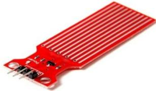
Fig:Water level Sensor
