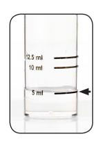
Add 8 drops of Ferroin Indicator (FE3144) and swirl to mix. The sample should turn orange.
