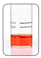
3 Add Nitrite Titrant (ND2272) one drop at a time while swirling. Count the number of drops until the sample color changes from orange to blue.
