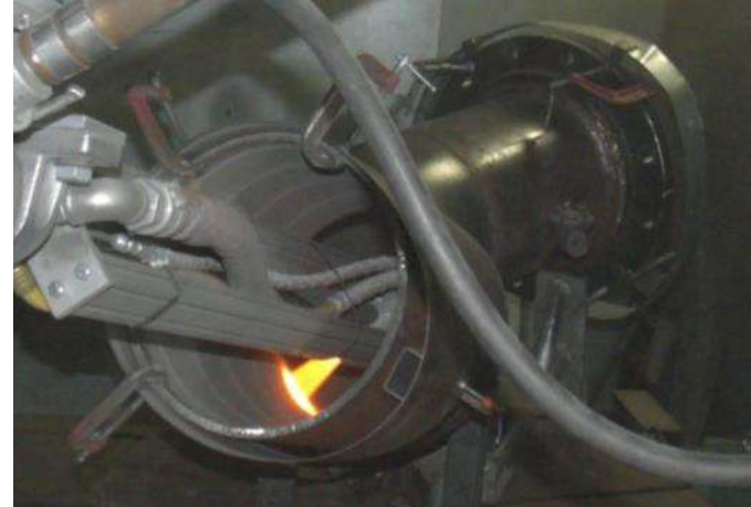
A Double Elbow Sprayed with our Rotating ID Gun
