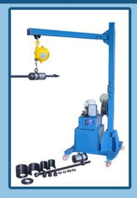
Single acting return hydraulic jacks are available in both alloy steel and aluminium, and have 50 and 100mm stroke which pin and bush can be replaced in one or multiple stroke. Jacks are center hole type and are placed on C-sleeves (one over the other) through which center rod passes and nuts are tightened at the ends. Tie rods and nuts are machined from an alloy steel material, hardened and tempered to increase strength and toughness.
