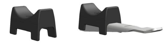
**Polymer Cable Saddles** are made from injection molded glass-filled Polymer resin to create a strong, non-conductive cable saddle for use with underground cable support arms in vaults and manholes. The fiber-reinforced polymer saddles are non-corrosive for long-term durability. Emits no harmful smoke. Secures the cable tightly to the saddle.
