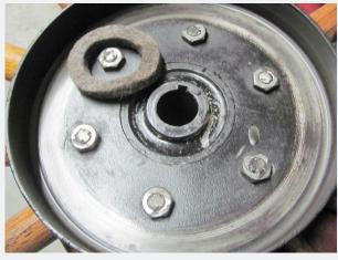
To install the seal, first rub a good coating of grease into the dry felt seal on the outside, as shown below. This holds the felt fibers together and provides lubrication. Compressing the felt while greasing makes it easy to place within the groove.
