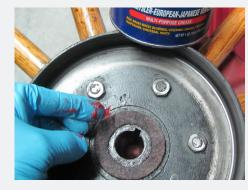
When the wheel is back on the car, the felt seal will ride on the axle housing cap, which is the outer seal for the Hyatt bearings. The photos below were taken after driving for hundreds of miles. In the photo on the left, the outer cap is a modern neoprene type seal and you can see its surface is now shiny from the felt seal revolving with the hub. In the picture on the right, notice the excellent condition of the felt seal inside the wheel hub after revolving on the outer cap.
