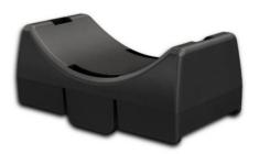
**Polymer Cable Insulator Saddles** are made from injection molded glass-filled polymer to create a strong, long lasting cable saddle for use with underground cable support arms in vaults and manholes. The fiber-reinforced polymer is both non-conductive and non-corrosive for long-term durability and emits low, unharmful smoke if exposed to fire. Two openings are provided at the opposing saddle tips for feeding the cable tie underneath the saddle, which secures the cable tightly to the saddle.
