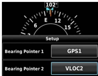
Figure 2-19 Bearing Pointer Setting
