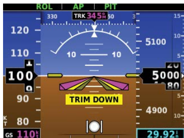
Figure 3-23 TRIM DOWN Alert
