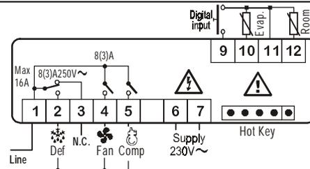
**NOTE:** The compressor relay is 8(3)A or 16(6)A according to the model. **120Vac supply:** connect to the terminals 6 and 7.
