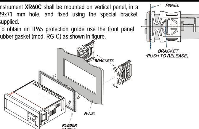
The temperature range allowed for correct operation is 0÷60 °C. Avoid places subject to strong vibrations, corrosive gases, excessive dirt or humidity. The same recommendations apply to probes. Let air circulate by the cooling holes.
