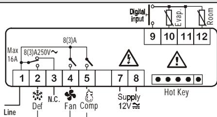
**NOTE:** The compressor relay is 8(3)A or 16(6)A according to the model. **24Vac/dc supply:** connect to the terminals 7 and 8.
