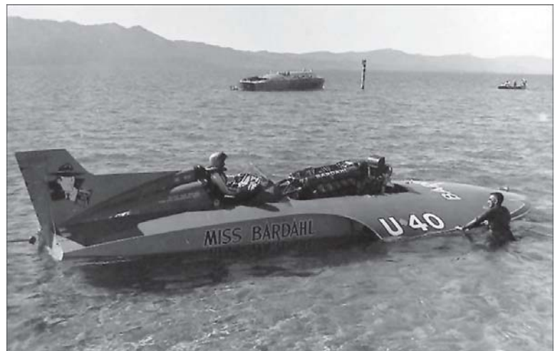
A crewman is pushing Miss Bardahl away from the beach and into deeper water so Ron Musson can start the engine without the propeller hitting the bottom and tearing things up. ~ Gene Patty photo
