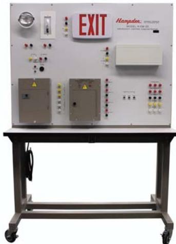
The **Model H-EM-2D** includes the following: Load Center, Control Console, Nickel-cadmium Battery, Battery Charger, Distribution Panel, Remote Control Alarm, Exit Sign Fixture, Flood Light and Wall Fixture.
