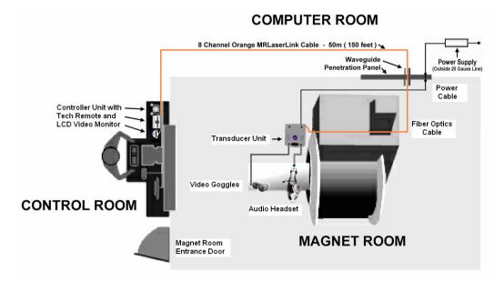
**Computer/Equipment room** Transducer is connected to power and fiber optic to transmit to the goggles and headset.
