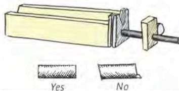
Clamp a block of wood against the pin and drill at the point where they touch.
