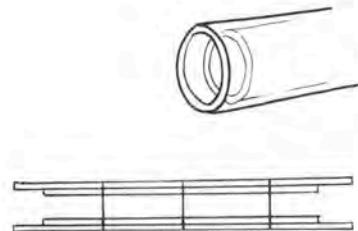
3. You will need several strips of flat springy metal. Watch mainsprings are best, but in a pinch, hard-drawn brass, or nickel silver can be flattened out and used. Cut two or three pieces about an inch longer than the hinge. Slide these through and lock them with a pair of wedges, tapped into place.
