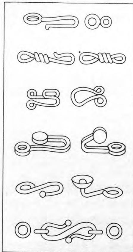
**19-11 HAND-FABRICATED HOOKS MADE OF WIRE, USED FOR CLOSINGS.**
