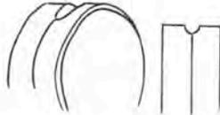
2. Buy or make two tubes that telescope together. Remember that soldered tubing can be drawn like wire, so it's pretty easy to get a good fit by drawing the tube through a drawplate.
