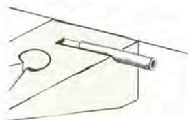
5. Burn off any residual glue from Step #3 and tie the box and lid together with binding wire. Prop it so the hinge groove is conveniently angled, apply a small amount of flux, and set the knuckles in place. Lay a tiny bit of hard or medium solder against each knuckle and allow the flux to dry.
