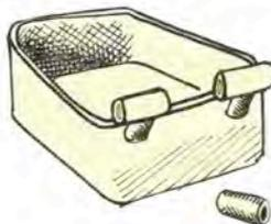
4. Solder a wire onto the lid, eyeballing its relationship to the other arms. In most designs, you'll be able to adjust this later. Solder a piece of the same tubing (larger than the gap) onto the end of this wire.
