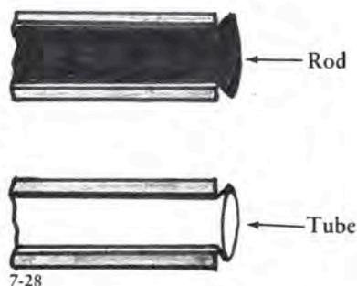
7-28 Hinge pin of tubing or rod.
