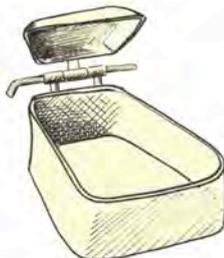
6. Bend the arms with pliers to make the parts work together. When the fit is right, some designs will benefit from the addition of strengthening supports.
