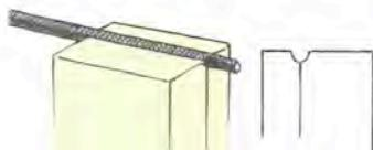
4. Clean the tube with Scotch-Brite to remove any finger oils and tarnish. Measure the length of the hinge and divide this into three or five parts. Set a tube cutting jig to this dimension and saw off the knuckles with a small sawblade. Inspect for burrs, and remove them with careful filing.
