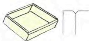
3. Secure the parts with glue or tape and convert the angled opening to a rounded one (e.g., change a "V" into a "U"). A tapered needle file can do the job, but a parallel round file is much better. An alternative is to find a steel rod (nail) with the same diameter as the hinge tube. Cut the end off square, mount this in a pin vise, and use it to scrape the groove.
