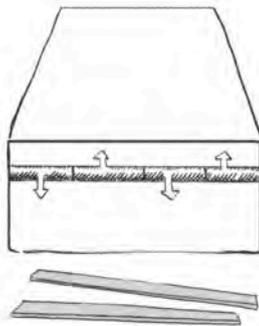
2. After polishing, slide a tight-fitting tube through the hinge to serve as the hinge pin, leaving it short by at least 3 mm on each end. This will provide strength and smooth operation. Skip this step if the hinge is small.
