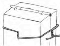
6. Gently heat the unit until the flux becomes crusty, then concentrate heat on one side. Bring this up to temperature, easing off as the solder starts to soften. Pull the heat away the instant the solder flows. Repeat on the other side. If you are not certain that the solder has flowed, resist the temptation to give it just another second. Resist!
