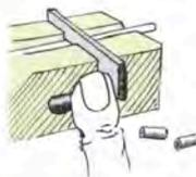
8. Set a knuckle into the cradle and solder it into place. Visually line this up with the center of the box.
