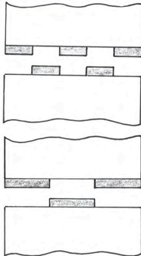
7-20 Sequence in which a three and five element hinge is soldered.
