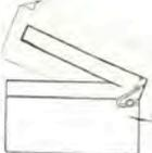
2. Drill a hole through the sides of the box and slide a length of tubing all the way through. File as needed to provide a snug fit.
