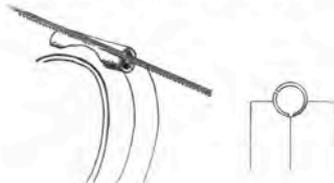
6. Make another cut, this time removing one-third of the tube. The result is a pair of cradles that are parallel, well-attached to both parts, and that fit the knuckles perfectly.
