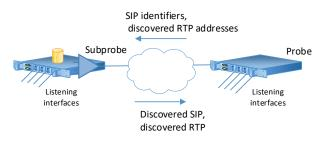
Here the VETap makes the decisions about which SIP packets to send to the probe. If the intercept provisioned in the probe specifies that the call media is also to be intercepted, the probe discovers the media attributes (IP and port addresses) and sends instructions to the VETap(s).
