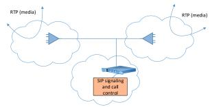
This might occur when there is a central part of the network where the SIP signaling is processed, and a probe could be placed there and listen to all the SIP traffic, but the media don't come to the central location and instead are handled in remotely dispersed gateways. Here the VETap subprobes are used at these remote sites to capture the appropriate media streams under the control of the probe.
