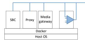
**VETap as a VoIP Subprobe**. The VETap software can be installed, along with Linux, in a server platform, and the configuration file can tell the VETap to tap certain of the server's network interfaces. Such a physical entity can be called a subprobe, truly a remote surrogate of the probe.
