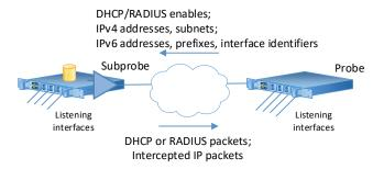
As the probe discovers dynamic IP address assignments to intercept targets, or if static IP addresses are being used for targeting, the probe provides the IP addresses (or subnets, etc.) to the VETaps.
